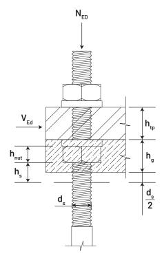
The resistance provided by the anchor bolts depends upon the anchor bolt steel, concrete strength and anchorage. If Anchor bolt's resistances cannot be transferred due to concrete failure, supplementary reinforcement to carry the forces must be provided.
