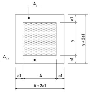
Required splitting reinforcement area
