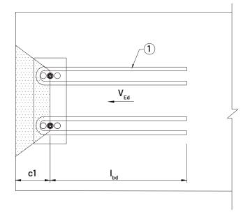
Table 26. Concrete Edge Reinforcement for SKP - L Type High Capacity Anchor Bolt
