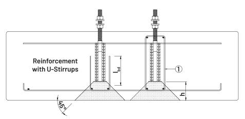
Table 28. Concrete Edge Reinforcement for SKP - L Type High Capacity Anchor Bolt
