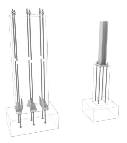
To increase the load-carrying capacity, anchors are assembled in a group. Moreover, this allows for a moment-resisting connection. For tension and shear load, the mechanical behavior is mainly influenced by
