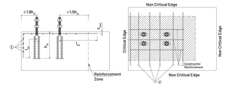
Table 22. Concrete Splitting Reinforcement for SKP - L Type for High Capacity Anchor Bar
